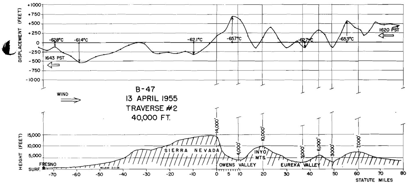
Fig. 4 — (Above) Mountain wave of 13 April 1955 as derived from temperature variations along the second 40,000 foot traverse of B-47. Note again the low point over the Eureka Valley and new wave excitation east of it. Tropopause close to 40,000 feet. Updrafts can barely support a glider. Max winds about 90 knots.
