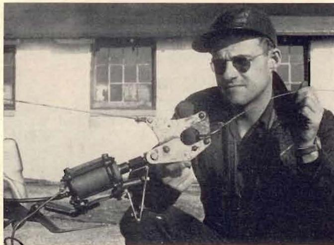
Fig. 1—The pressure cylinder. Art Heavener shows how the hinged cylinder stays in alignment with the tow wire. The string attached to the release can be pulled by the tow car operator in case of emergency thereby releasing the glider.
