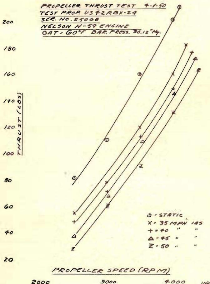
Fig. 7—The net thrust vs. RPM at various indicated air speeds for a representative test propeller.
