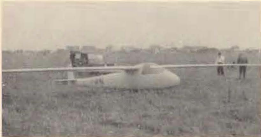
The very high aspect ratio and slender wing are apparent in the Italian designed and built SPILLO.
