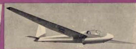
SGS 2-25: Two-place, high-performance sailplane. Flown in English Internationals, and set unofficial altitude record of over 43,000 feet in Sierra Wave Research Project.
