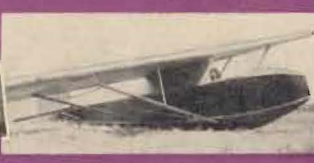
SGU 1-3: Larger span and plywood type fuselage were the new features of this trainer.
