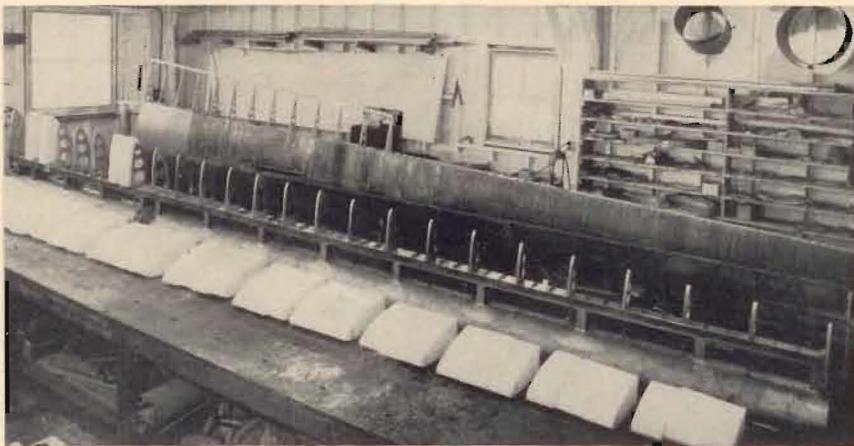
At this advanced stage of construction are shown the Styrofoam pieces cut to rough size. After insertion in the leading edge, they are contoured to shape.
