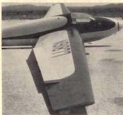
Here is the 1-23 with the extended wing-tip in position.
