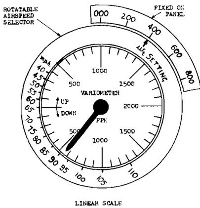
spacing between the "hundred feet per minute" units), the adjustable table can be made into a ring which can be set by rotating it to the appropriate  $w_t$  value. Then the one ring will be valid for all conditions.
