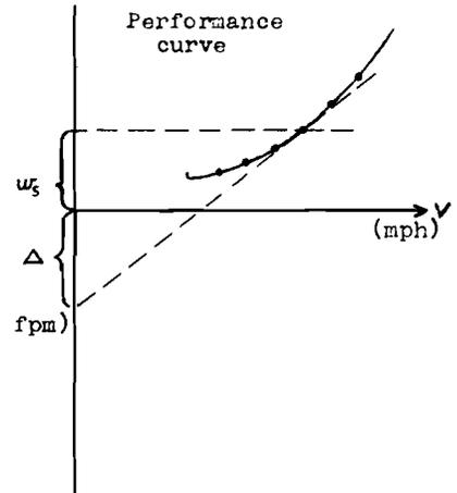
Step 1) Draw the performance curve of the glider ( $w_s$ , sinking speed, vs. velocity).
