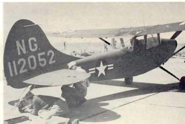
Pete Bowers tightens the nut holding the hook on the L-19's tailwheel while Heasley Entz strings the release line. Note superior cabin visibility. (See story on page 9)
