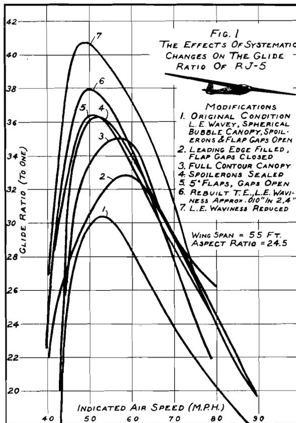
in this manner permitted the maximum glide ratio to be raised from 30 to 1 to 40.5 to 1. Fig. 1. A similar gain on a transport airplane would raise its cruising range 30%.
