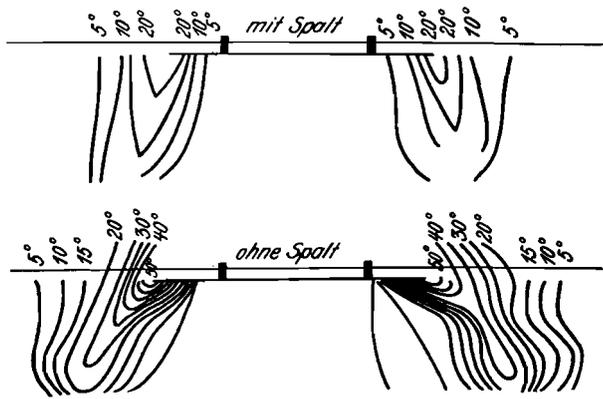
Fig. 5. Curves of equal deflection from undisturbed flow. Above, with a gap under the spoiler, and below, no gap.
