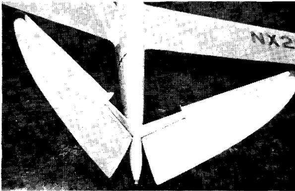
Vee type tail surfaces stick forward rudder neutral
