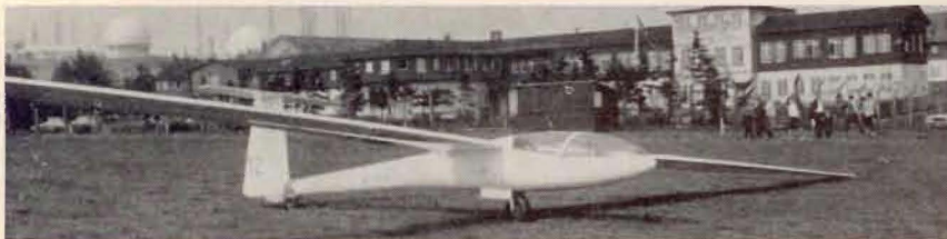
L/D—48:1 @ 62 mph • Min. sink—1.6 ft/sec @ 45 mph • 2 m/sec sink at 110 mph U.S. Deliveries starting April 1967 — Contact your nearest Schleicher Dealer.
