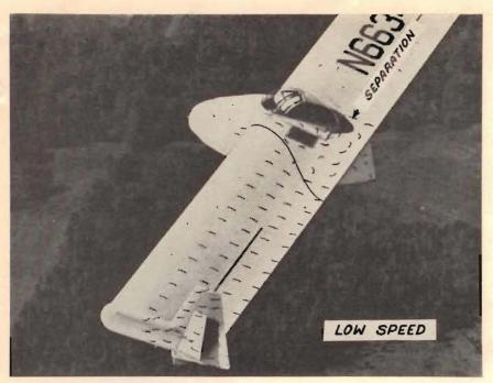
The separation on the upper surface will have its largest effect in the low speed range since it will reduce the lift and span efficiency factor. The separation in the lower surface intersection will reduce the high speed performance as it represents an increase in drag. No tufts were used on the bottom of the pod but an area of separation is expected aft of the wheel. Also it was found that the forward part of the tip fins were ineffective.
