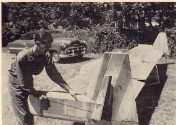
Jock Powell demonstrates the action of the drag flaps at the tip fins.
